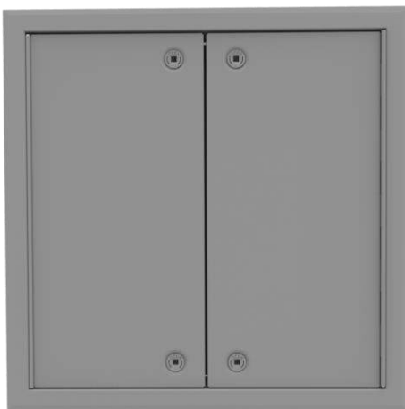
APM – Double Door Metal Access Panel with flanged edge, piano hinge and square cam lock.
